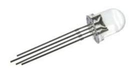
The goal of the task of creating a program is to read one at the start of the program and then set the diode to that color. You will need to use PWM to be able to control the diode correctly. It may be that you have to implement the PWM function yourself in your application, or does Arduino come with useful functions? Use suitable inputs / outputs to control the diode. The LED should light up with the set color until the program ends.
